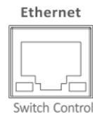
**Remote Port :** Control the switcher RJ-45 Female connector
