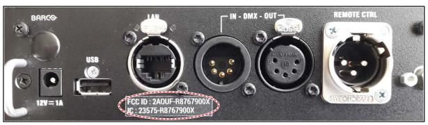
Image 7-8 Example of the black label on the communication board
