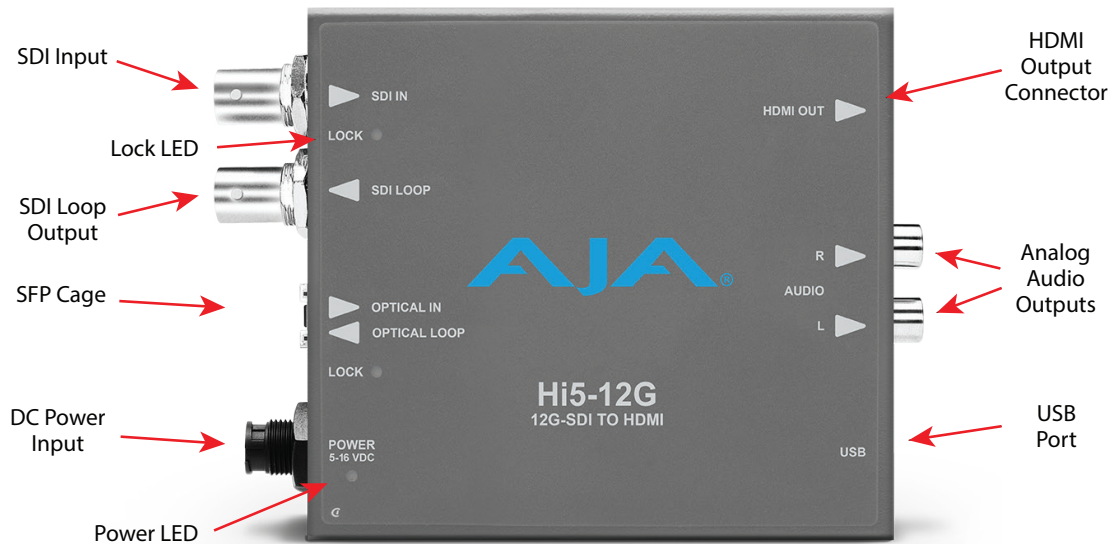
Figure 2. Hi5-12G Converter Connections
