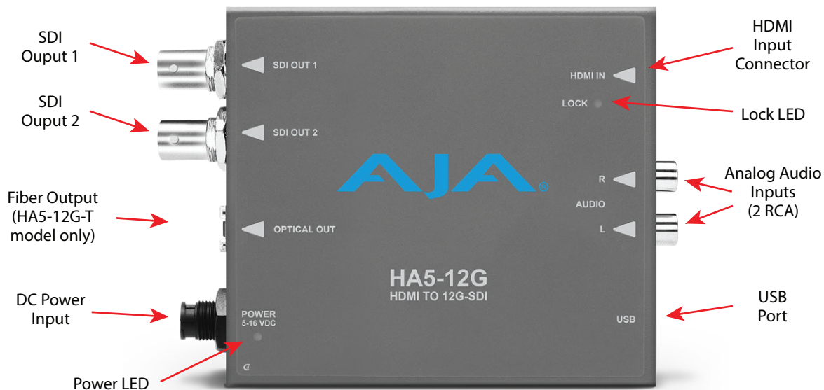
Figure 2. HA5-12G/HA5-12G-T Converter Connections
