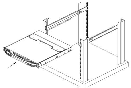
4. Slide the rear attachment sliding brackets along the slide bars until they contact the rear of the CL3800, then use the screws supplied with this package to attach the bars to the rear of the CL3800 (tighten the screws all the way).
