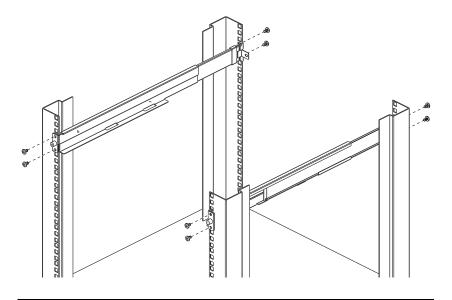
3. Slide the CL3800 onto the support flanges. Use the screws supplied with this package to loosely attach the front of the CL3800 to the front of the rack (only tighten the screws part way).
