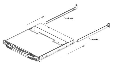
2. Attach the left and right *easy-installation* mounting rails to the inside of the rack. The flange that supports the CL3800 will be to the inside.
