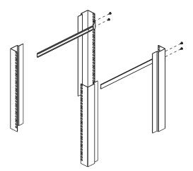
2. While one person inserts the CL3800 into place by sliding its left and right side bars into the mounting brackets (on the rack), have a second person install four screws in the front tabs to secure the module to the front of the rack.
