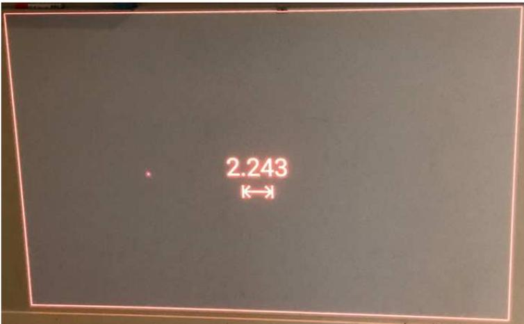
Image 8-8: Example of projected image during laser ranging session with measurement on screen
