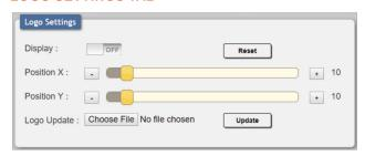
This tab provides control over the user uploaded logo graphic. Controls include positioning, an uploading a new logo directly from the WebGUI and an option to reset the logo to a built in default image that can be used for testing.
