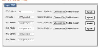
This unit provides the option of three standard EDIDs, two sink sourced EDIDs and four user uploaded EDIDs that can be assigned to all inputs at the same time, or to each input independently.
