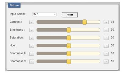
This tab provides controls over each input's contrast, brightness, saturation, hue, and sharpness levels.
