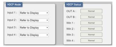
This tab provides control over the HDCP settings for all inputs.
