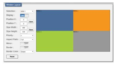
This tab provides control over the position, size, aspect, priority, and other settings of each window in multi-viewer modes. A graphical representation of the layout is also provided. When the unit is in Matrix mode, only a limited selection of controls are available.
