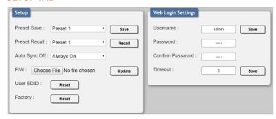
Provides a way to update firmware and reset various sections within the unit. Control over the unit's Auto Sync Off feature, storing/recalling presets as well as configuring the WebGUI login settings is also provided here.
