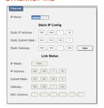
This tab provides controls to change the network settings for the unit. You can manually set the IP address, netmask and gateway address in "Static IP" mode, or you can obtain an IP address automatically by enabling DHCP.
