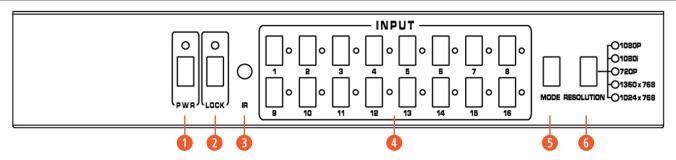
**1 POWER:** Press this button to power the device ON/OFF. The LED will illuminate Green when the power is **ON**, Red when it is in **'Standby'** mode.
