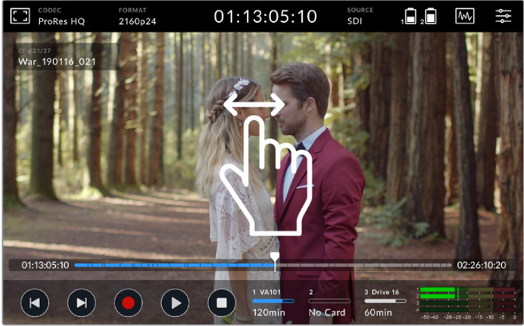
On Blackmagic 12G HDR jog forwards or backwards by swiping the video left or right.
