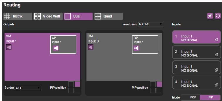
Figure 27: The Dual Tab – PIP Mode
