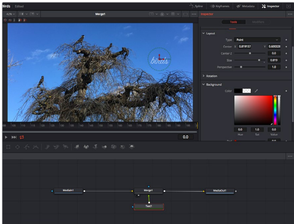
Selected nodes appear with a red border. Here the inspector panel is displaying the layout tab controls for the text node.
