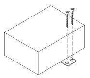
For installation on a drywall surface, use a #6 drywall screw. When installing, it is recommended to thread the drywall screws into a stud.
