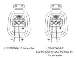
Figure 8: Subwoofer polarity with LC2-PC30G6-8/LC2-PC60G-8H/LC2-PC30G6-8L
