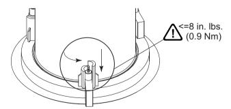
Figure 10: Tighten mounting tabs
