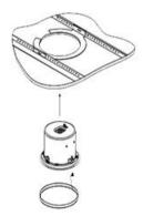
Figure 9: Mount speaker into ceiling
