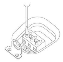
Figure 6: Tighten with screwdriver
