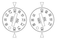
**Figure 12:** Adjust tap selector (left: LC2-PC30G6-4/LC2-PC30G6-8/LC2-PC30G6-8L; right: LC2-PC60G6-10/LC2-PC60G-8H
