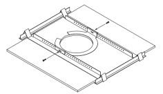
Figure 5: Secure rails to C-Ring
