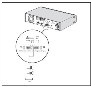
figure 4.3: Connecting speakers
