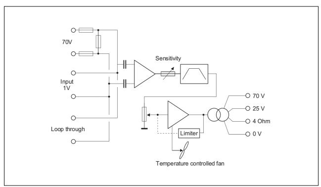
figure 2.1: Schematic overview of the Plena Power Amplifier
