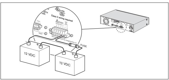
figure 4.1: Connecting a DC power supply
