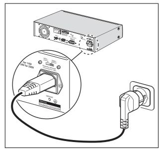
figure 3.2: Power connection and voltage selector
