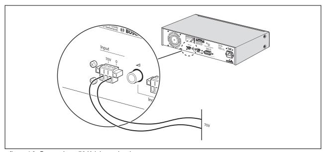
figure 4.2: Connecting a 70 Volt input signal
