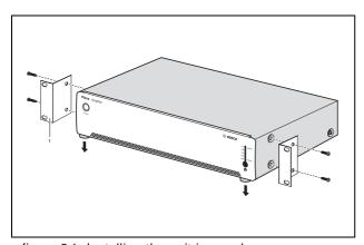
figure 3.1: Installing the unit in a rack
