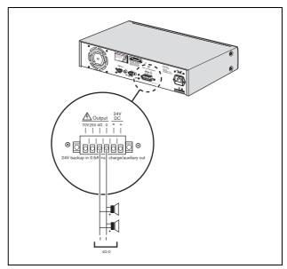
figure 4.4: Connecting speakers
