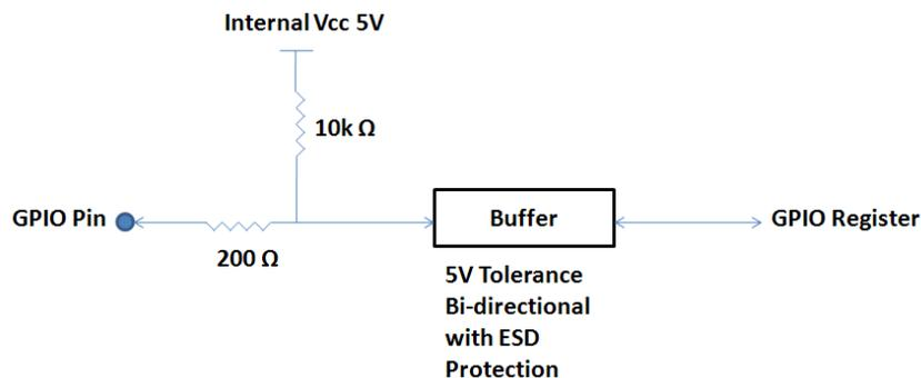
Figure 4-8: GPI/O Electrical Characteristics
