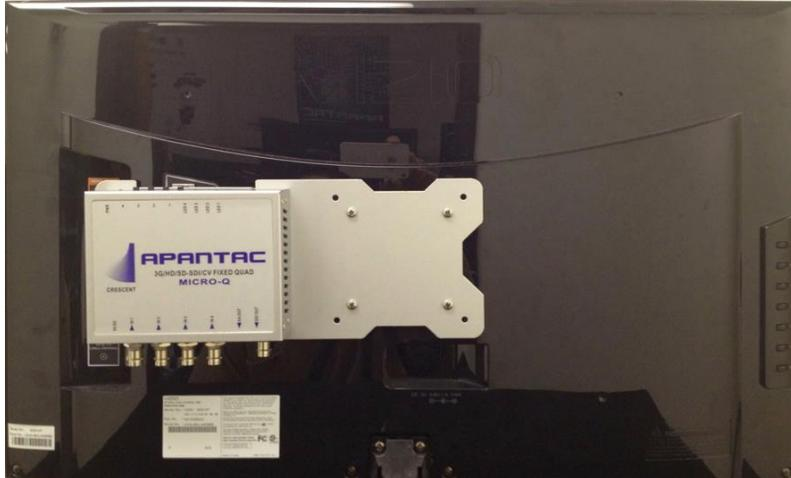
Figure 4-3: MicroQ Optional VESA Mounting Plate with MicroQ
