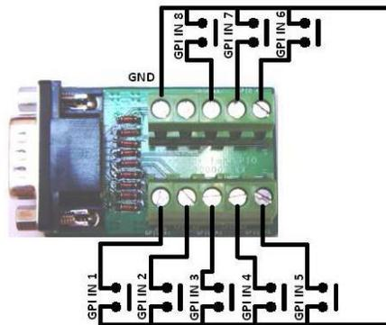
Figure 4-7: Wiring diagram for GPI inputs
