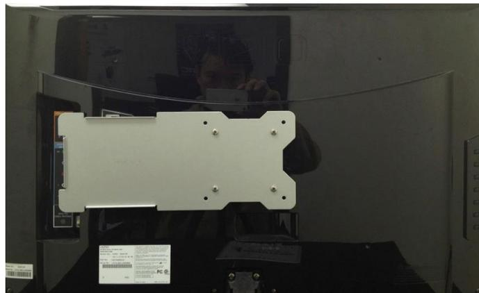
Figure 4-5: MicroQ Optional VESA Mounting Plate
