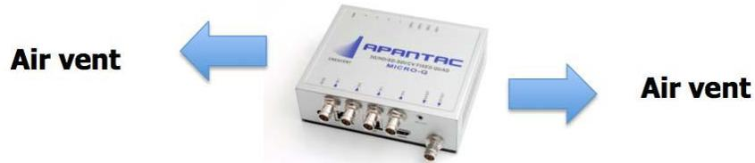
Figure 4-3: MicroQ Venting
