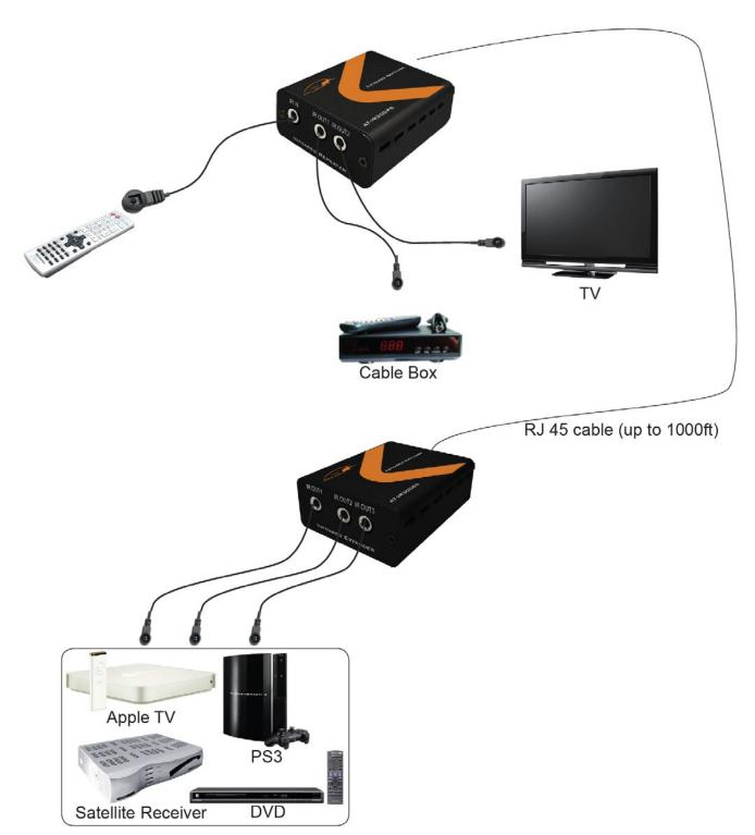
Note: IR receiver eye can take signals from up to 20 ft. away in the open distance
