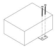
For installation on a drywall surface, use a #6 drywall screw. When installing, it is recommended to thread the drywall screws into a stud.
