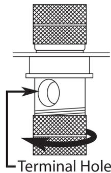
3. For each terminal insert the corresponding positive (+) speaker wire into the terminal hole on the screw terminal with the red stripe, then turn the sleeve clockwise to secure the wires.
