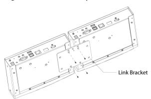
3. Remove the bottom and side screws from each unit.
