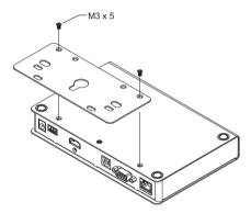
3. Screw the mounting bracket to any convenient location on the rack.
