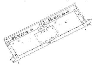
4. Screw the mounting brackets to the rack.
