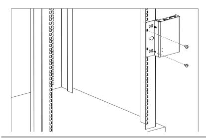
**Note:** Rack screws are not provided. We recommend that you use M5 x 12 Phillips Type I cross recessed type screws.
