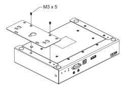
3. Screw the mounting bracket to any convenient location on the rack.
