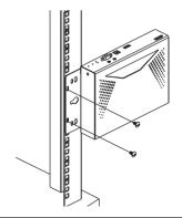
**Note:** Rack screws are not provided to mount the unit. We recommend that you use M5 x 12 Phillips type I cross screws.
