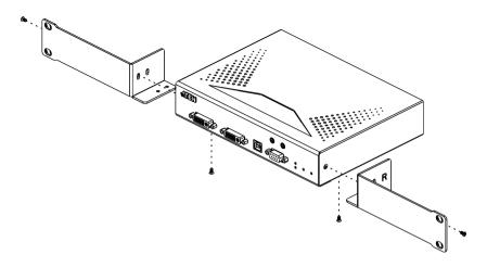
4. Screw the mounting brackets to the rack.
