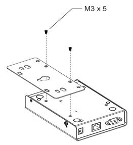
2. Use the center hole to screw the bracket to a secure wall surface.
