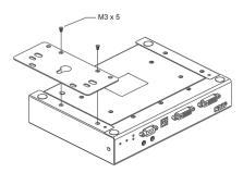
3. Screw the bracket into a convenient location on the rack.
