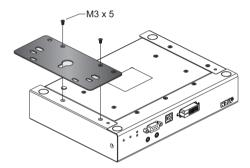
3. Screw the mounting bracket to any convenient location on the rack.
