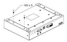
2. Use the screws from step 1 to screw the mounting bracket to the bottom of the unit.
