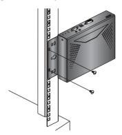
**Note:** Rack screws are not provided to mount the unit. We recommend that you use M5 x 12 Phillips type I cross screws.
