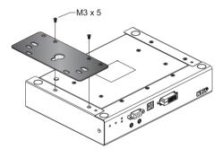
3. Use the center hole to screw the bracket to a secure wall surface.
