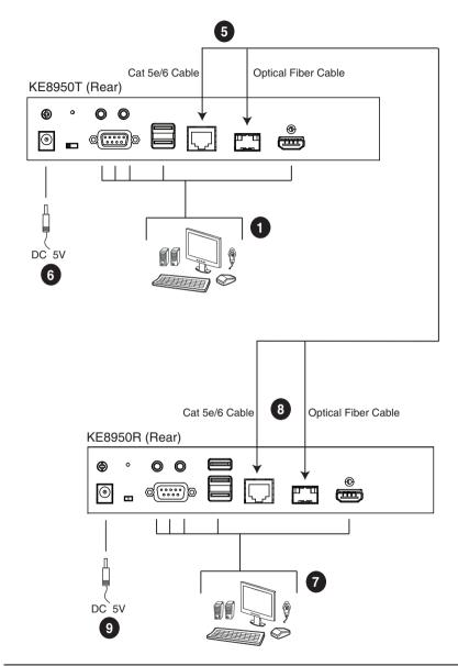
**Note:** Power adapters are not provided with the KE8952. Please contact your ATEN dealer to purchase additional power adapters, or use the Power over Ethernet (PoE) feature to supply power to the KE8952.
