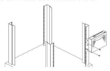
**Note:** Rack screws are not provided. We recommend that you use M5 x 12 Phillips Type I cross recessed type screws.
