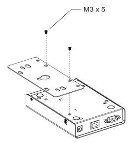
2. Screw the bracket into a convenient location on the rack.
