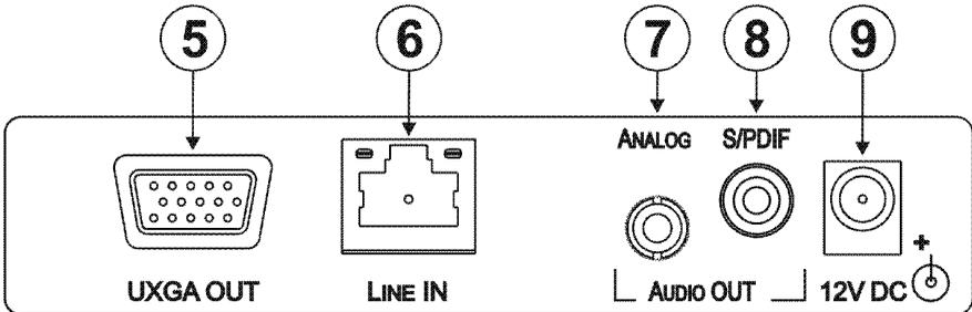
Figure 4: TP-122xl UXGA/Audio Line Receiver Rear Panel
