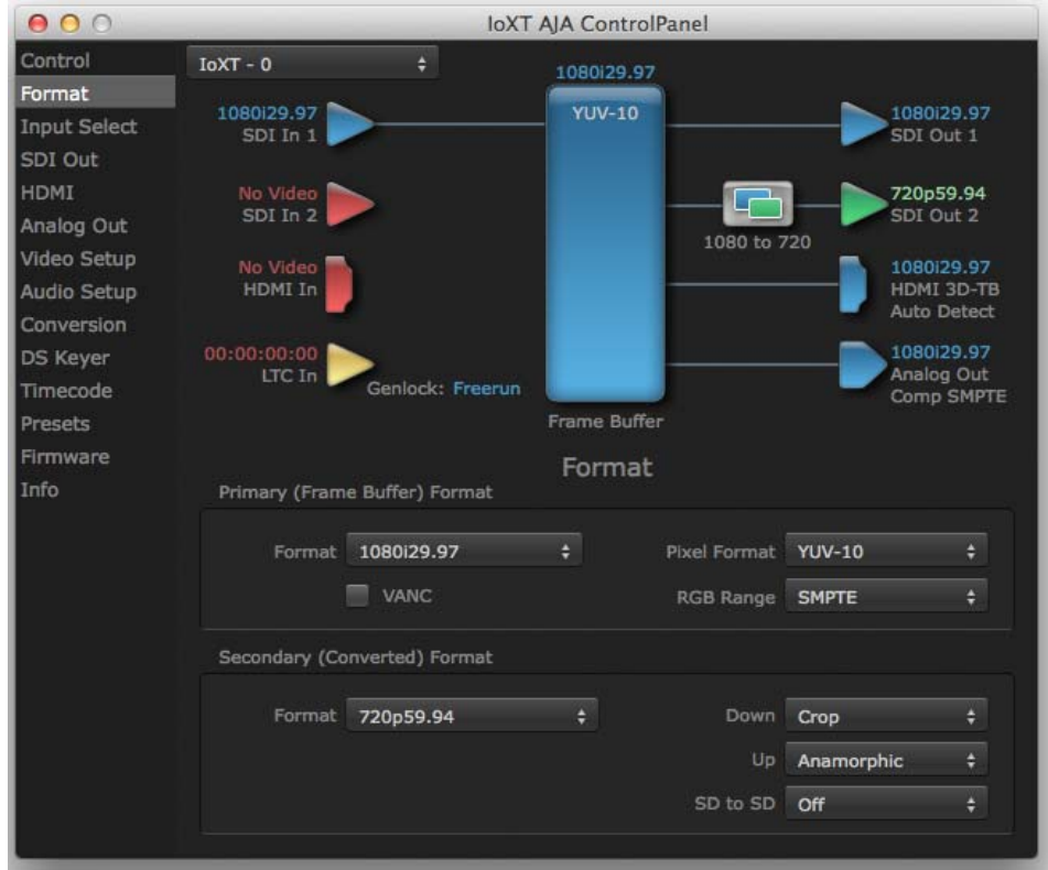
Figure 28. AJA Control Panel, Formats Screen, Example shows Io XT cross-conversion
