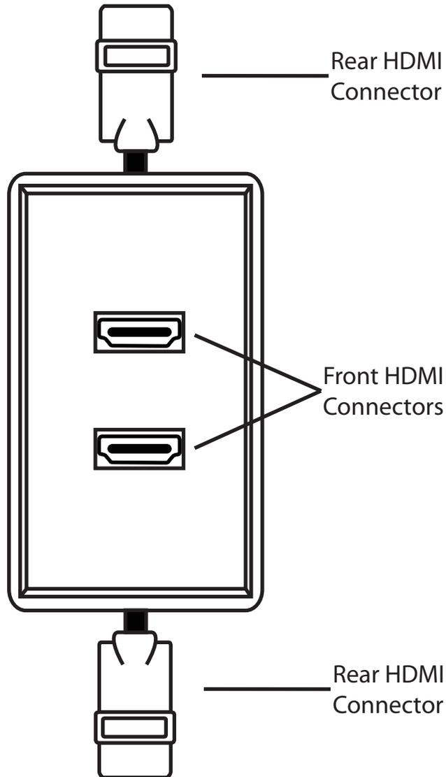
3. Remove the Face plate from the wall plate by pushing down on HDMI connectors with your thumbs and at the same time pulling two opposite corners away. Under the face plate you will find two screws hidden there. Place the wall plate against the opening of the electrical box, then thread the two supplied screws through the screw holes in the wall plate and the electrical box, then tighten the screws and reattach the face plate.
