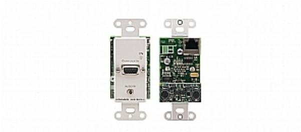
The WP-301xl is a wall plate twisted pair transmitter for computer graphics video & stereo audio signals. The unit converts the input signals to a twisted pair signal that is converted back to the original signals by a compatible Kramer receiver.
