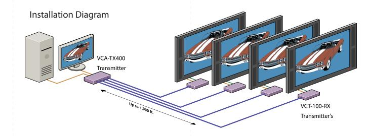
VCT Transmitter Installation Diagram
