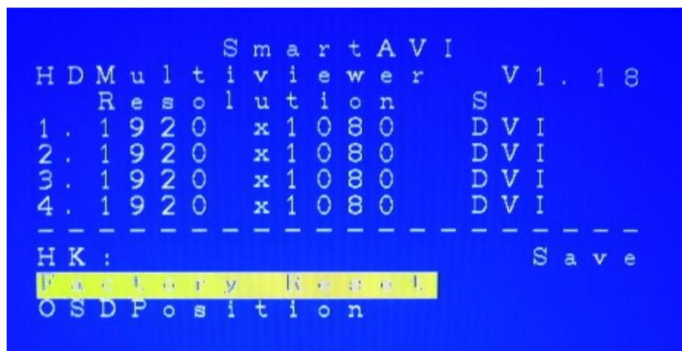
The position of the OSD can be moved around. Select the “OSD Position” text and press enter. Next use the up, down, left, and right arrows from the keyboard to move the position of the OSD. Likewise the 1, 2, 3, 4 buttons on the front control panel will move the OSD as well where 1 is down, 2 is up, 3 is left, and 4 is right.
