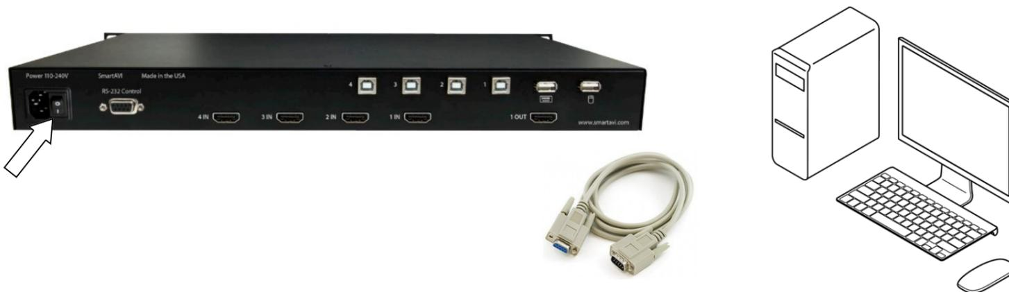
Next connect to the device using HyperTerminal or a similar serial data application and an DB9 for RS-232 connection. The settings for the connection are as follows:
