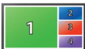
**PiP Mode** - In the PiP (picture in picture) mode, the full screen displays one of the four video sources, and is accompanied by three smaller images (thumbnails) containing the other video sources on the right-hand margin of the screen, allowing simultaneous monitoring.
