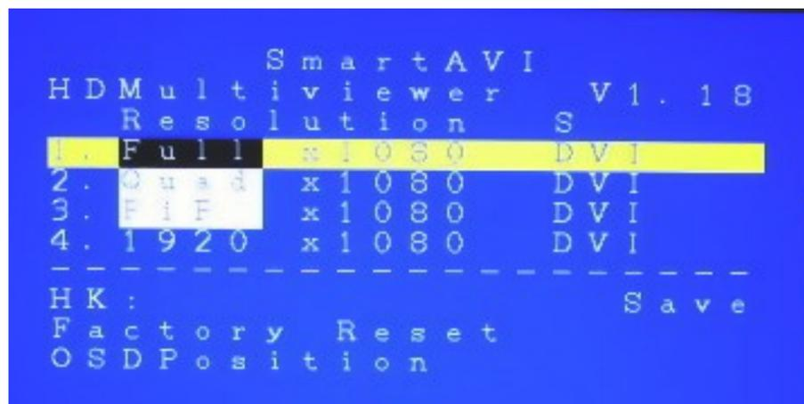
The hotkey can be changed by using the up and down arrow in the OSD and pressing right arrow on “HK:” Next, a submenu will come up with the option to change the hotkey to ctrl, shift, and alt.
