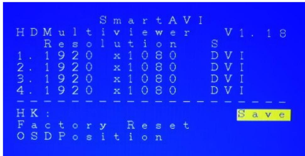
To restore the factory settings click scroll down to “Factory Reset” and press enter. The HDMV will perform a power reset on itself.
