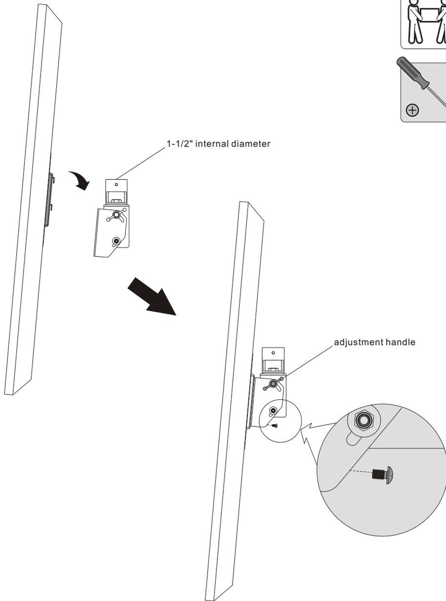
Hook the VESA plate (attached the display) onto the ceiling mount head and tighten the screw to secure it.
