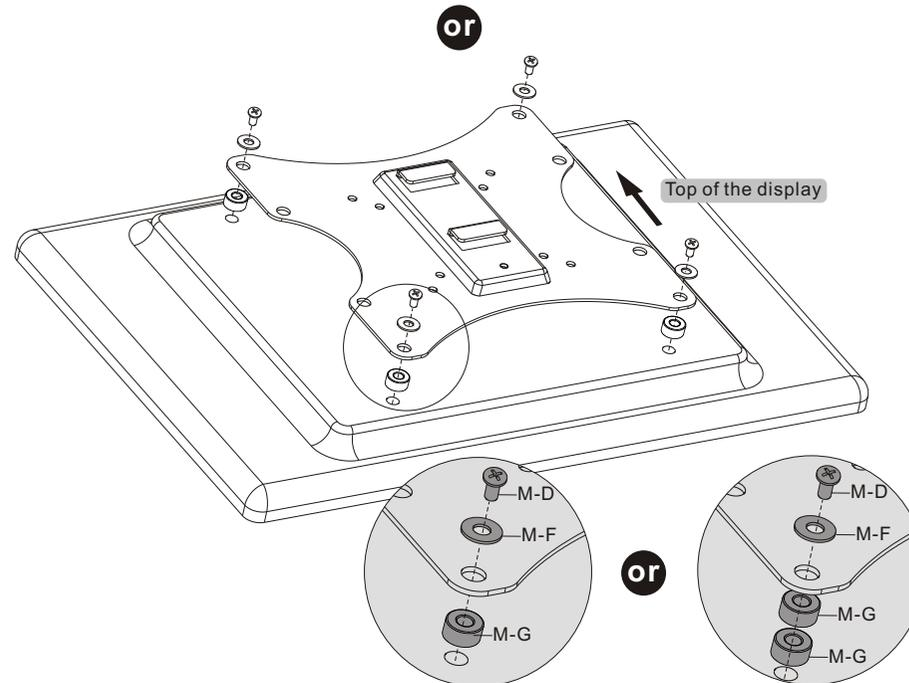
**Note:** Choose the appropriate screws, washers and spacers (if necessary) according to the type of screen. Screw the VESA plate onto the display.
