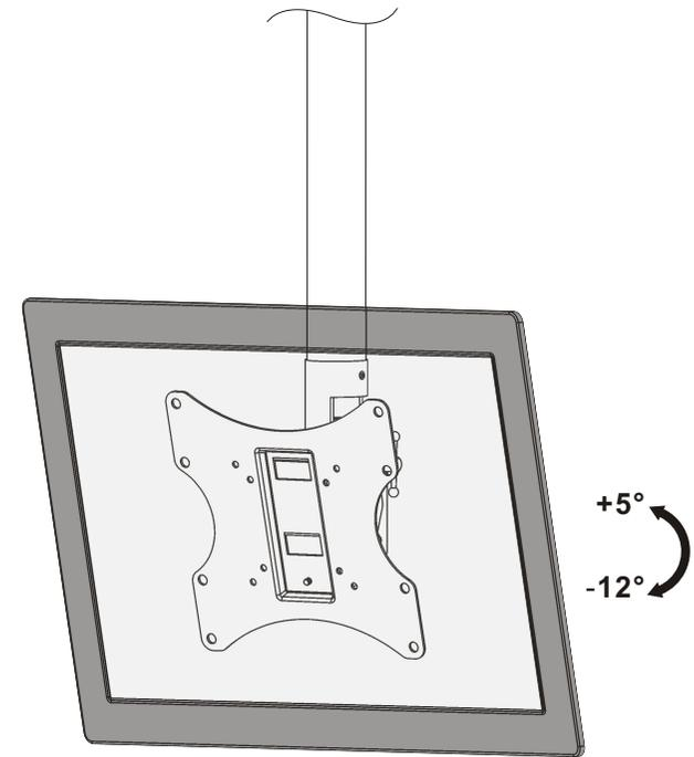
Loosen the adjustment handle to adjust the display to obtain the desired angle then tighten it.
