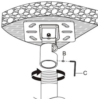
Insert and tighten one set screw to secure it.
