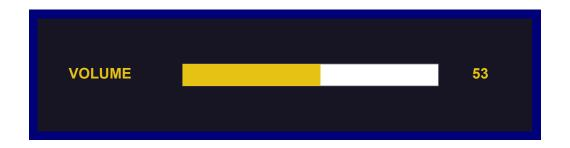
Press ▼ button on the monitor first, and then press - / + buttons to adjust volume on the monitor.
