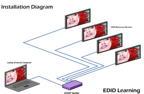
The Display Data Channel (DDC) is a digital connection between a computer display and a graphics adapter that allows the display to communicate its specifications to the adapter.
