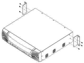
3. Position the device in the rack and align the holes in the mounting brackets with the holes in the rack.
