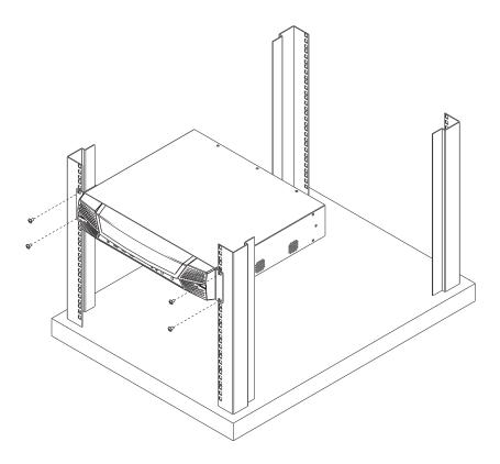
Note: Cage nuts are provided for racks that are not pre-threaded.
