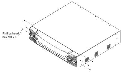
2. Use the M3 x 8 Phillips head hex screws supplied with the rack mount kit to screw the rack mounting brackets into the front of the unit.
