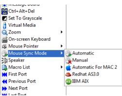
• Linux doesn't support DynaSync Mode, but there is a setting on the Mouse Sync Mode menu for Redhat AS3.0 systems. If you are using a USB Adapter Cable (see the Note on the previous page), with an AS3.0 system and the default mouse synchronization is not satisfactory, you can try the Redhat AS3.0 setting. In either case, you must perform the manual mouse synchronization procedures described in the next section.
