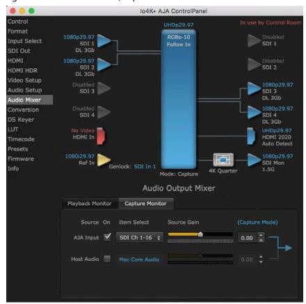
Figure 11. Audio Mixer Screen, Capture Monitor Mode
