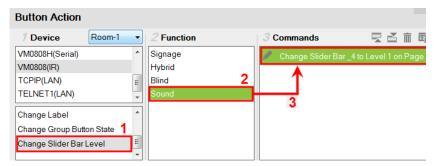
4. Double-click **Change Slider Bar** in the *Commands* list and use the drop-down menus to select the **Slider Bar** and **Level**.
