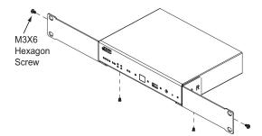
3. Screw the mounting brackets to the rack.
