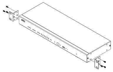
2. Position the unit in the front of the rack and align the holes in the mounting brackets with the holes in the rack.
