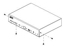
2. Use the two bottom screws removed in step 1 to secure the bottom of the brackets, and two M3X6 hexagon screws (from the rack mount kit) to secure the side of the bracket to the VK1100.
