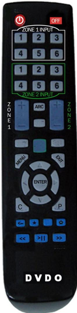
**Power and Standby/Off** buttons are discrete functions and can be learned into any universal remote.
