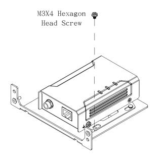
4. If the video extender doesn't have a mounting bracket, align the bottom holes and then screw the video extender to the mounting plate.
