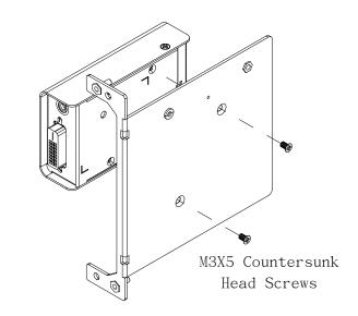
5. Slide a 3U Mounting Plate with video extender attached onto a slot in the VE-RMK3U Frame, aligning the screw holes and fitting the notches. Secure the mounting plate to the frame with two Plastic
