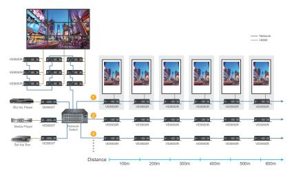
Use daisy chains to configure a video wall or expand the AV system hundreds of meters
