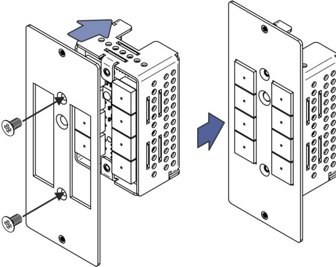
Figure 6: T-RC8IR Installation
