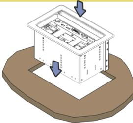
Secure the unit to the table and connect the cables.
