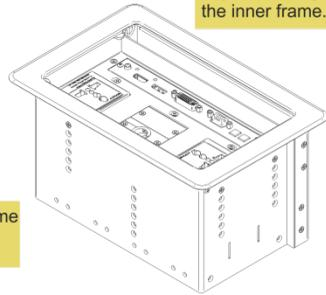
Mount the inner frame into the **TBUS-10xl** enclosure.
