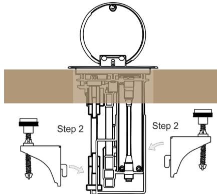
**Step 3:** Tighten the butterfly mounting screws securely upward against the table.
