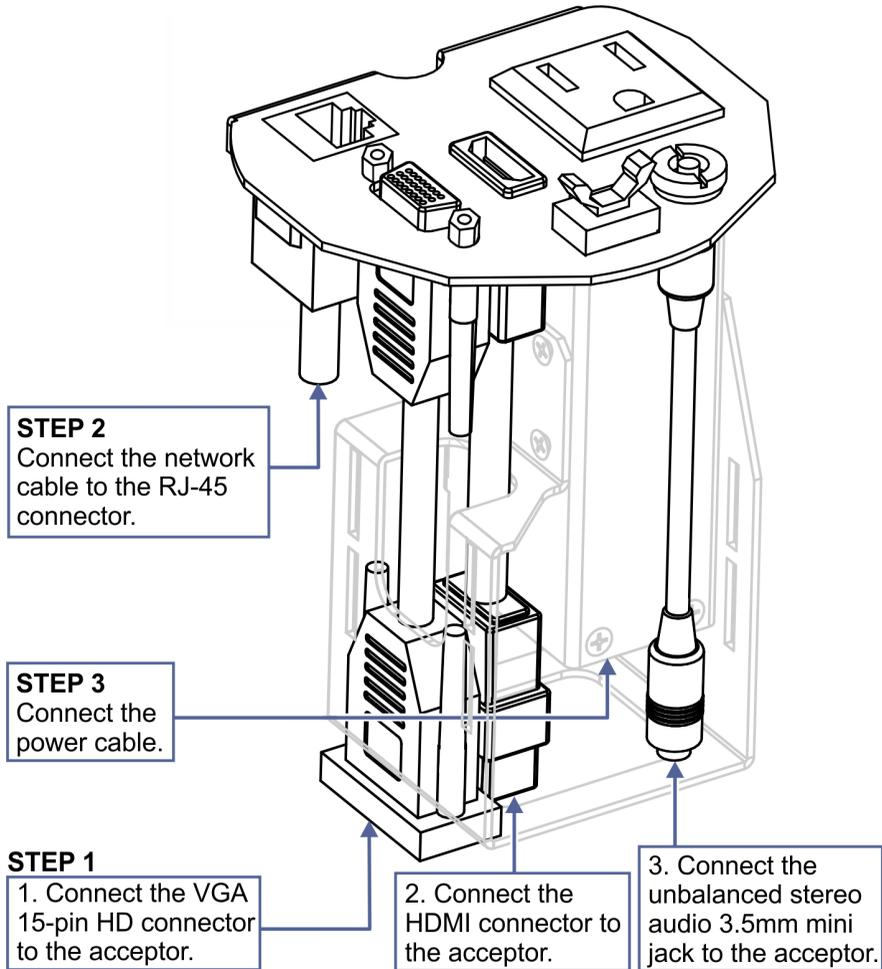
Figure 3: Connecting the Cables
