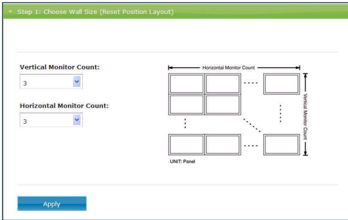
Figure 15: TV Wall Setup – Setting the Wall Size to 3x3
