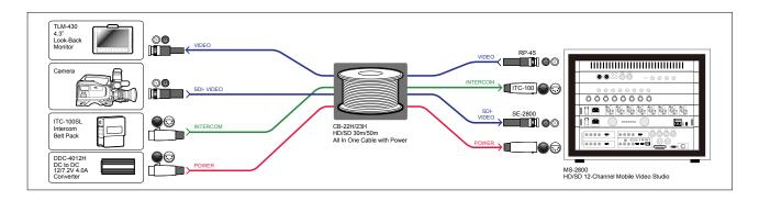
HD/SD 30m/50m 4-in-1 Cable for Multi-Camera Control (HD-SDI/ITC/CV/Cat-5)
