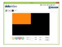
With a 4K input, you can define which part of the 4K input source to display. Just select the monitor number below, and drag and drop the color box to select the area to display. Or key-in the starting point by pixel, and press "Apply" to save changes.
