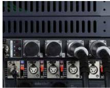
All-in-One cable is connected to the CCU-100 Four-Camera Control Center on the rack.
