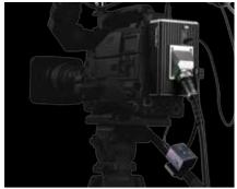
AD-2 is attached to the rear of the camera directly.
