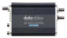
DAC-91 is an audio embedder that allows users to embed 2 channels of analog audio into an SDI video signal. It features 3G/HD/SD-SDI to support up to 1080p/60 video, automatically detecting and switching between different formats, and provides mini XLR and RCA audio connectors for inputting embedded analog audio.
