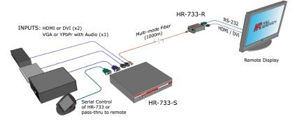
Figure 2 - Block Diagram (HR-731-S only has one HDMI video input)
