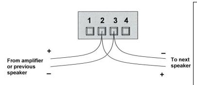
Figure 9 - Parallel Wiring
