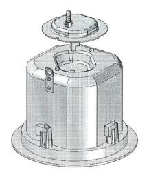
Figure 11 - Plug connector into connector socket
