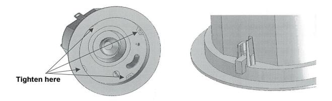
Figure 13 - Tightening the mounting tabs
