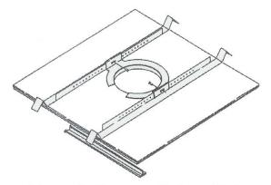
Figure 4 - Secure rails to split ring
