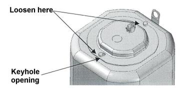
Figure 5 - Removing the strain-relief fitting
