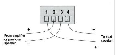
Figure 10 - Daisy-chain wiring
