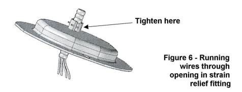
Tightening onto flexible or hard conduit - The supplied fitting accommodates up to 3/8 inch (9.5mm) flexible conduit. Insert the conduit into the strain relief fitting. Using the two horizontal screws that clamp the fitting together, clamp the conduit securely between them. Be sure to leave at least 4 to 6 inches of cable beneath the strain relief fitting.
