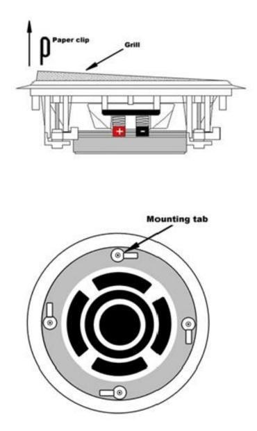
Be sure to position the four Mounting Tabs on your OWI speaker inward then insert the four (4) screws (supplied) from the front of the speaker into the screw opening.
