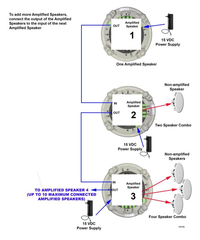
**One, Two, Four Speaker Combination Wiring**
