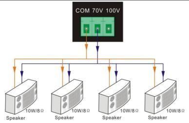
**Figure 4 Audio Output Connection**
