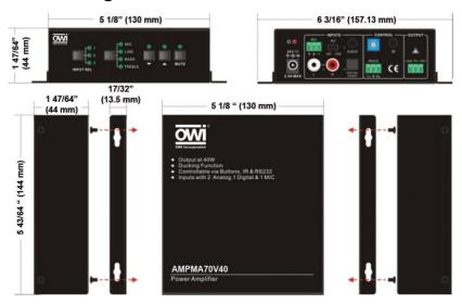
Figure 13 Panel Drawing
