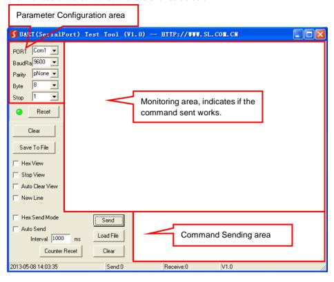
Figure 12 Main Interface of Control Software
