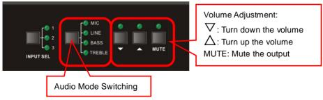
Figure 7 Audio Mode and Volume Adjustment buttons
