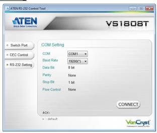
On the RS-232 Settings page, the serial port should be configured as follows:
