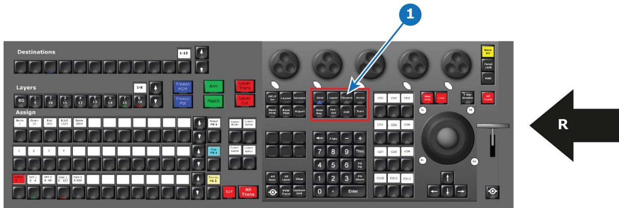
Image 10-21 1 Syntax entry Button Group R Right Side of the Controller
