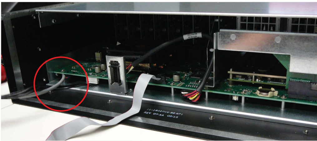
Image 14-35 USB Ext Cable connected to the Motherboard
