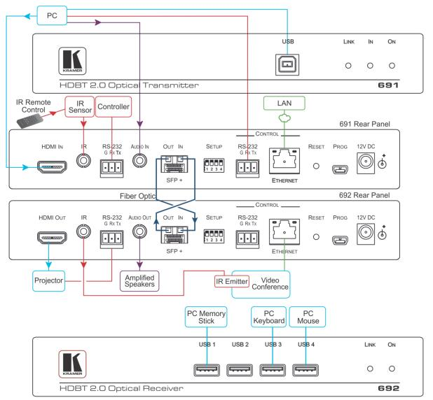
Always cross-connect the fiber connections, Rx OUT to Tx IN and Rx IN to Tx OUT, as transmission is carried on simplex fiber strands.
