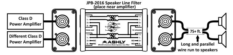
Another simple technique when routing long speaker lines from separate Class-D amplifiers is to leave some physical distance ( $\sim 2$  to 3 inches minimum) between each bundle run that is tied to each separate amplifier as shown below.
