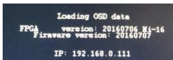
Figure 5: IP address of the unit will be displayed for about 5 seconds on boot up.
