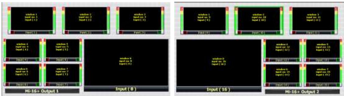
Figure 129: Preset9 – 9 windows with 2 audio meters and labels inside (Preset9.OPx)
