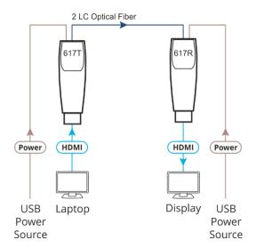
Once the system is connected the Status LEDs on both 617T and 617R flash.
